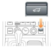
If single point entry has been used and only the driver's door is unlocked, the taildoor can be opened by pressing the release switch.
